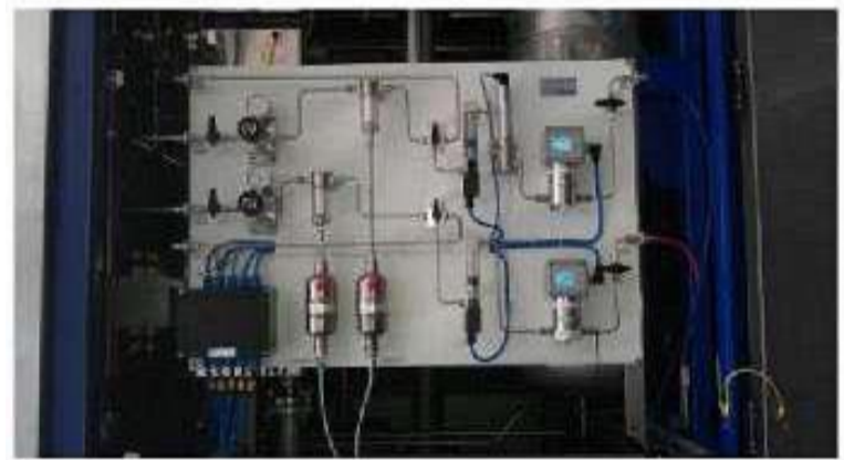
Panel with aerosol Trap for pressure electrolyzer 50 bar
