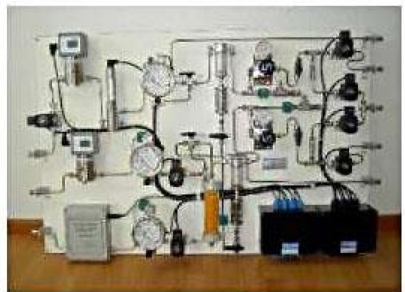
Panel O2 in H2 and H2 in O2 SIL for Pressure electrolyzer 30 bar
